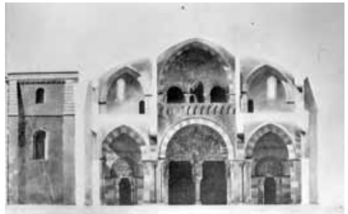
Figure 190. Viollet-le-Duc, La Madeleine, section of the porch with proposed restoration (1840)
