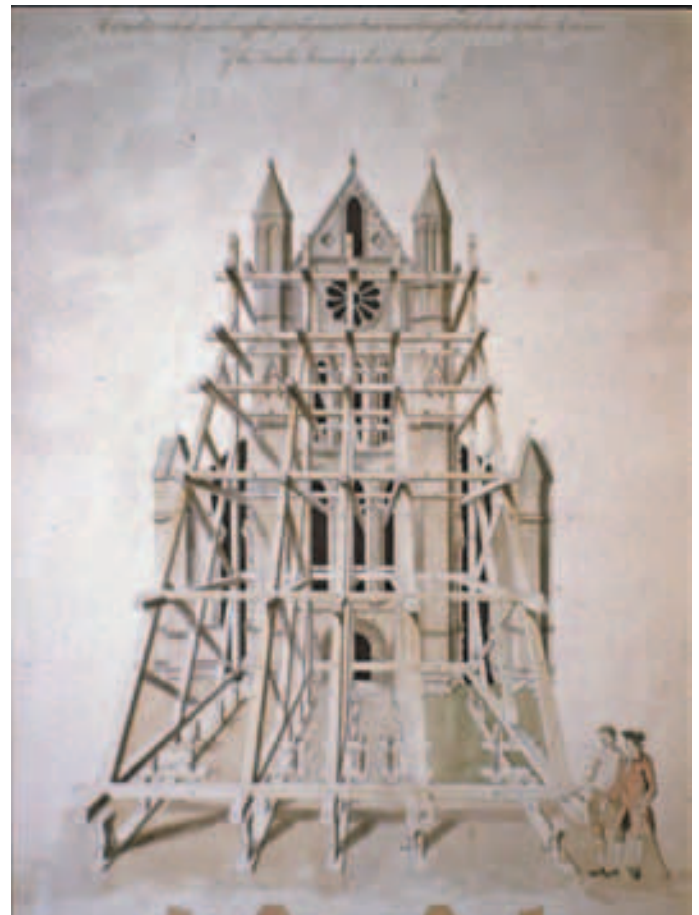
Figure 61. Beverley Minster, north transept. Drawing by N. Hawksmoor for a wooden machinery to push the leaning front back in position
